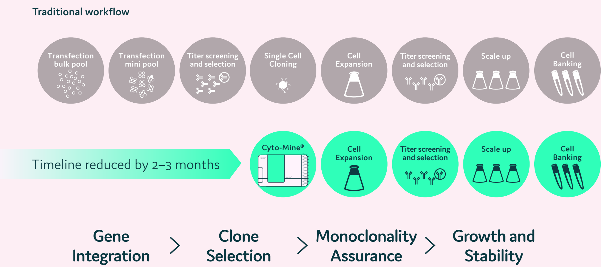
Figure 3: Traditional CLD processes are time-consuming. Cyto-Mine ® reduces time and increases success rates. At a single cell level, the clones are selected based on their productivity. Selected single cells are dispensed into microplates with image assurance on their mono-clonality. Cells dispensed into microplates can be monitored for growth over time.
